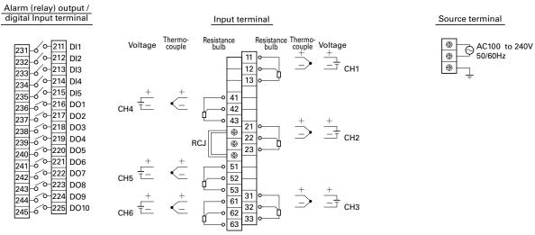
(Note1) For current input, connect an optional shunt resistance to a voltage input terminal.
