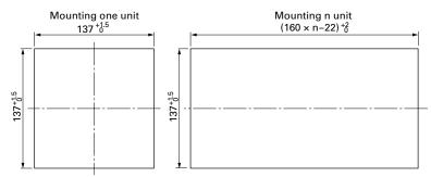
Do not use the water proof packing in case of mounting n unit
