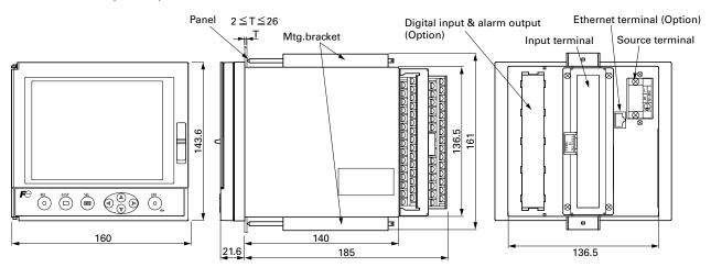
(Note) When placing the main unit on another instrument or on the floor, allow a space of 100mm or more between the unit and instrument or the floor.
