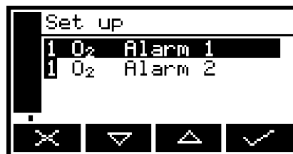
Figure 27: The Alarm set up screen
