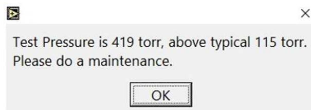
Figure 69: Pump Pressure Failure
