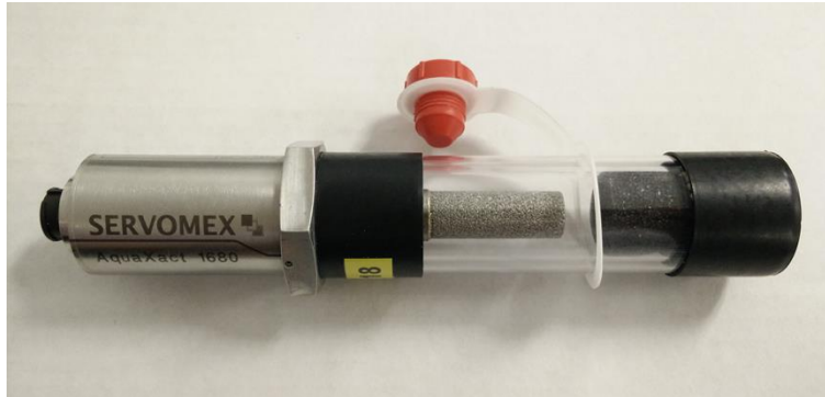
Figure 9-1: AquaXact 1688 Al 2 O 3 sensor glass storage bottle
