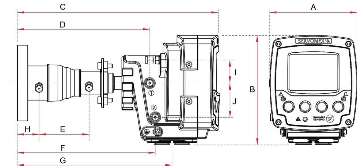
Figure 2-6: Transmitter unit dimensions
