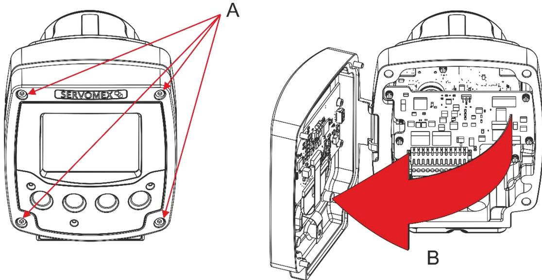
**Figure 7-17: Opening the transmitter unit**
