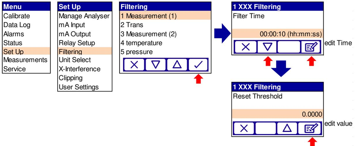
Figure 4-26: Filtering configuration menu
