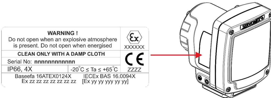
Figure 1-2: Laser 3 Plus receiver unit certification label location
