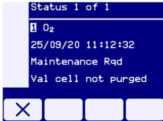
The reason for raising this status flag is safety related. If the cell is not purged properly then on exit from auto validation it may still contain span-gas. This could result in the analyzer producing an incorrect process measurement. There would be no other fault or anything to let the user know that the measurement may not be correct.
