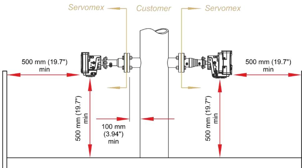
Figure 7-1: Laser 3 Plus installation distances
