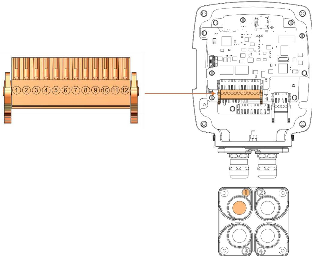
Figure 7-21: 12-way options board connections
