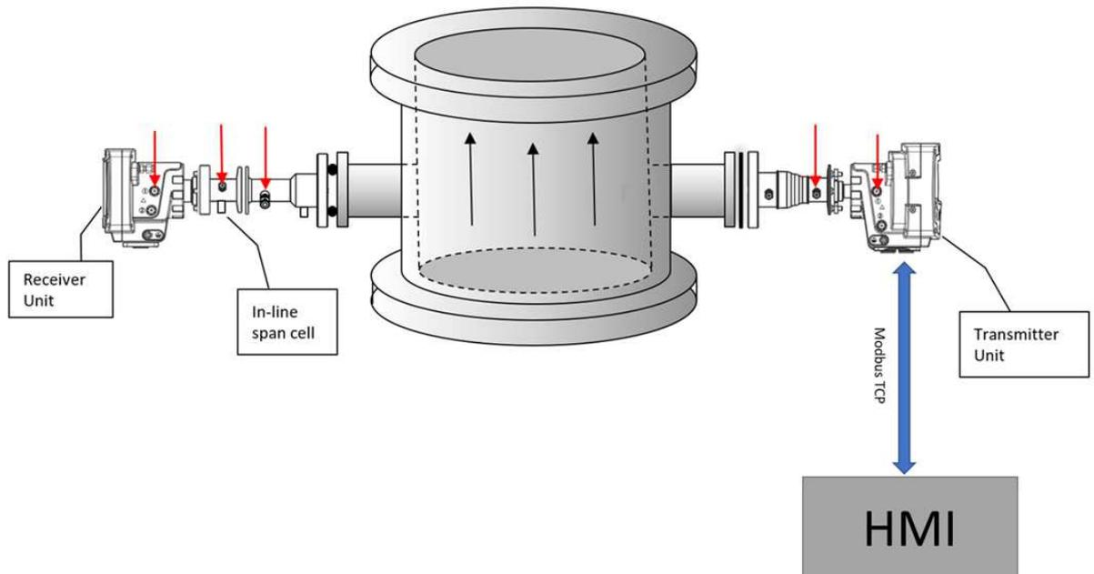
As shown in the diagram, communication between the Laser 3 Plus and the HMI is via Modbus TCP. There is a two-way flow of data between the Laser 3 Plus and the HMI.
