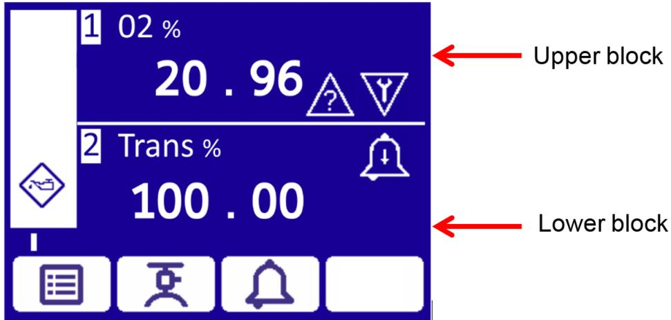
To assign a measurement reading to upper and lower display blocks
