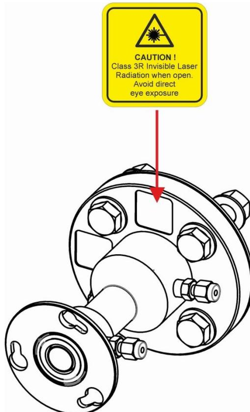
**Figure 1-6: Laser 3 Plus mount laser label location**
