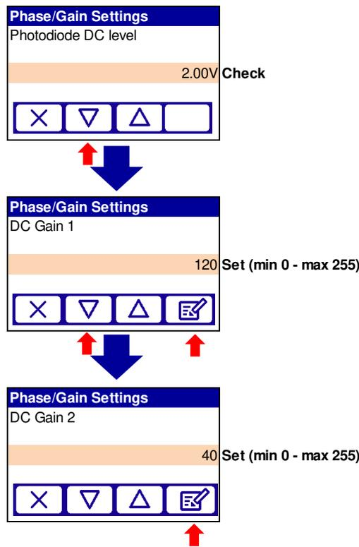
**Figure 4-32: Adjust gain and phase menu**
