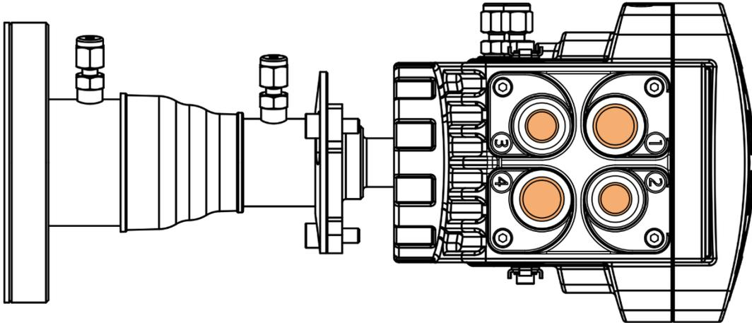
**Figure 7-16: Transmitter unit cable gland positions**
