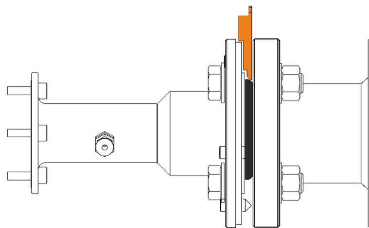
**Figure 7-27: Installation: Large O-ring initial setting**
