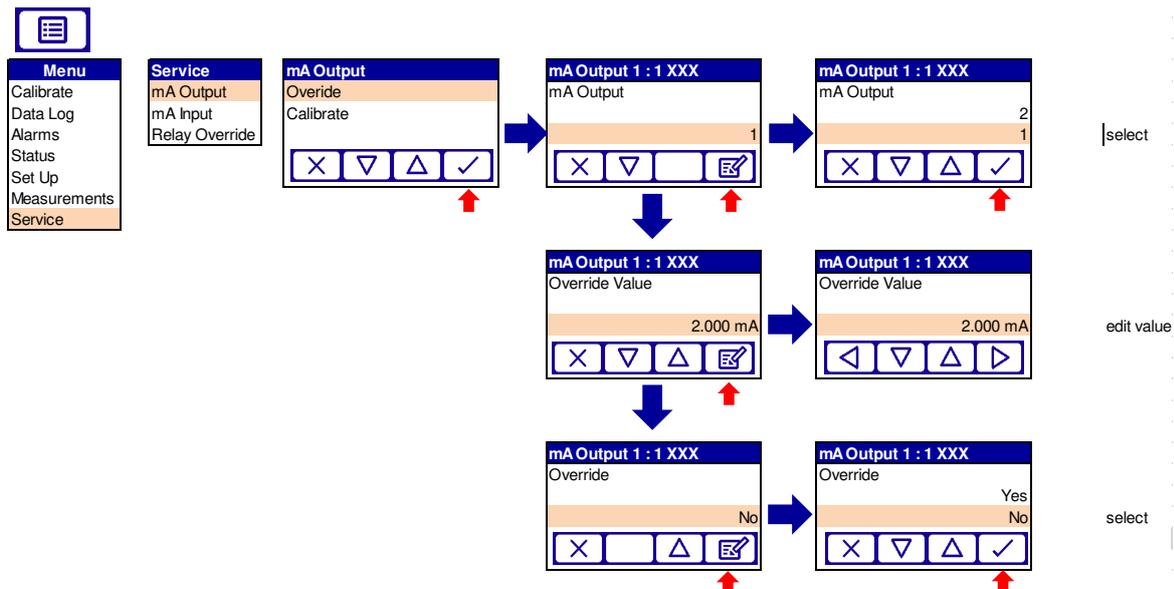
**Figure 4-14: mA output calibration and override menu**
