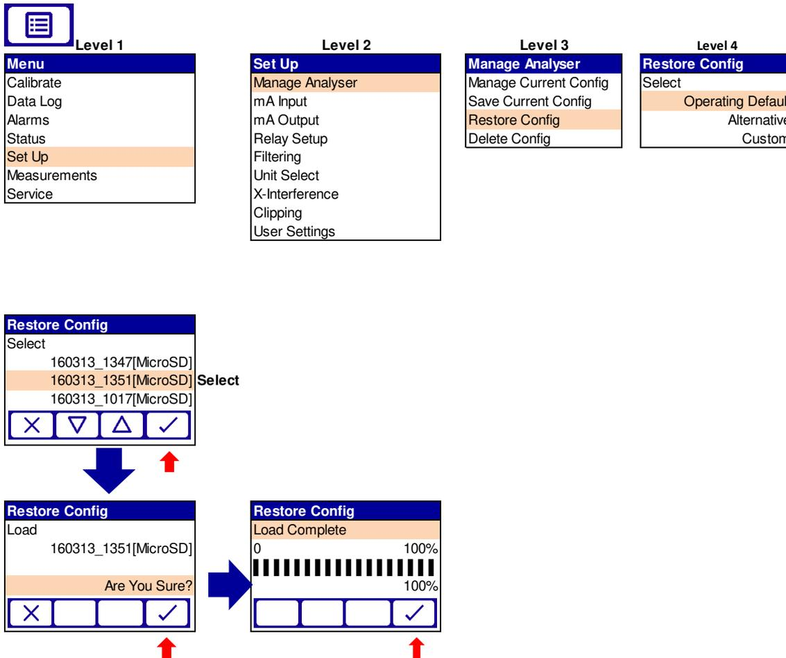
Figure 3-9: Restore measurement (detailed) settings
