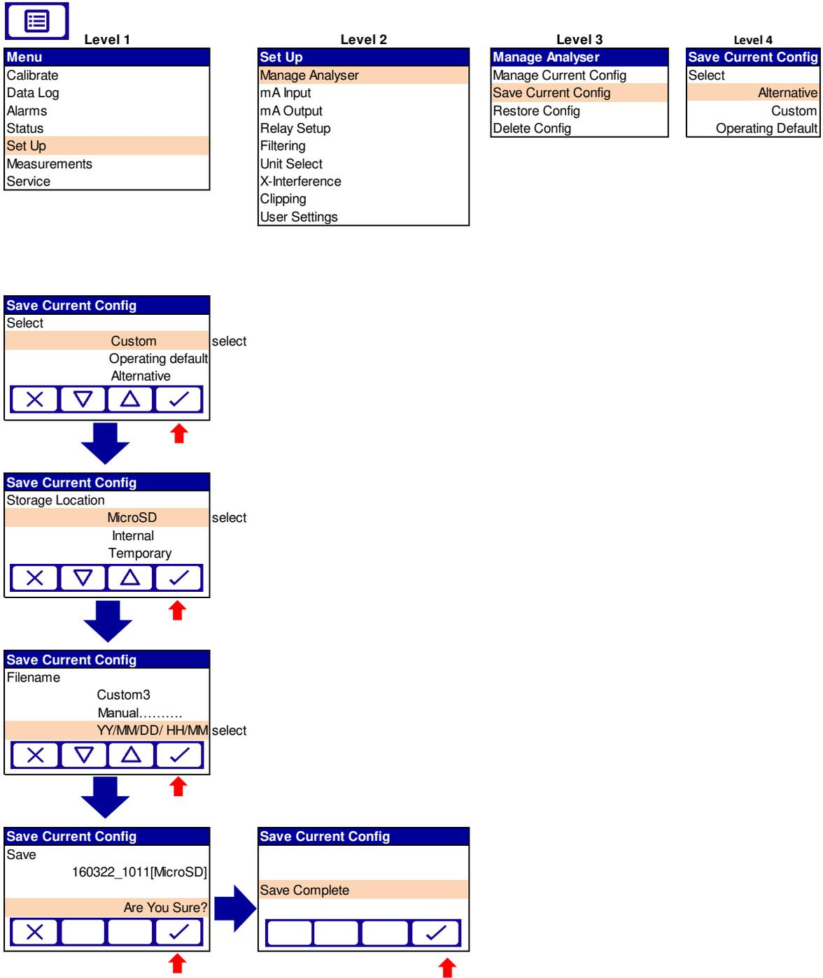
Figure 3-8: Saving sensor measurement (detailed) settings
