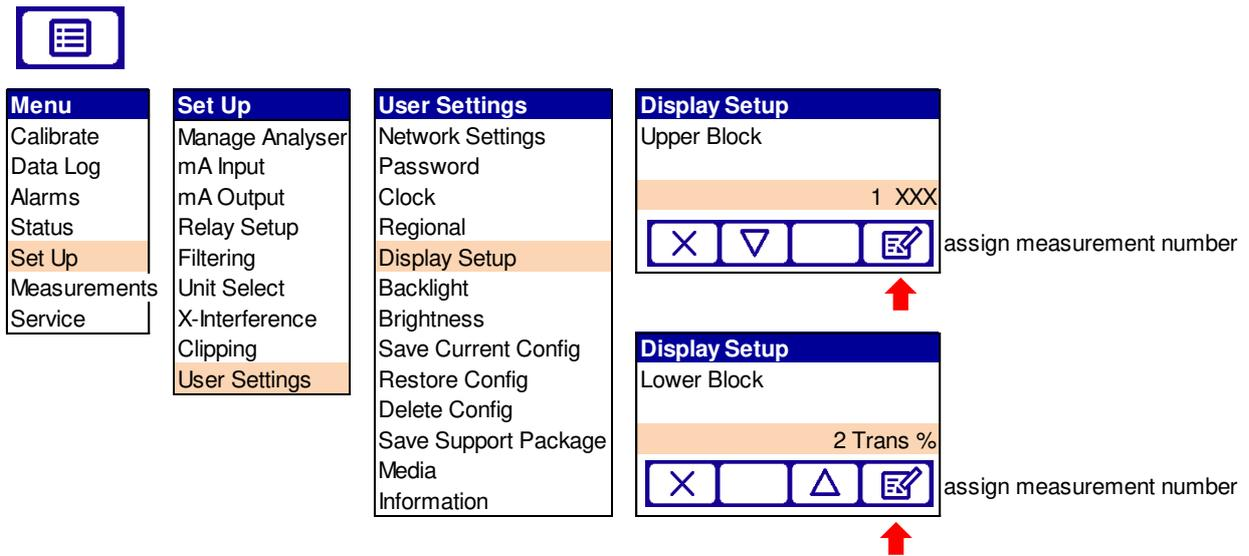
Figure 4-4: Upper and lower display block menu
