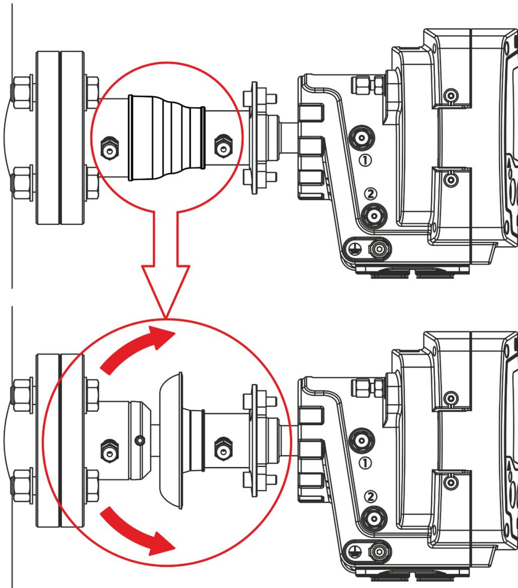
**Figure 7-24: Peel back the boot**
