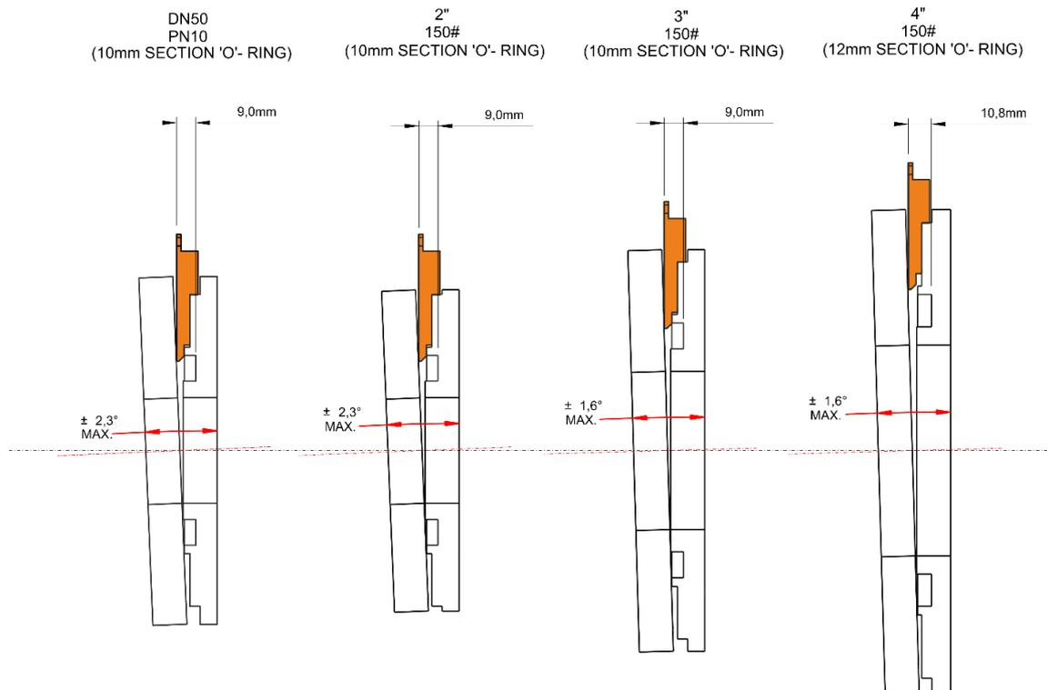
**Figure 7-28: Installation: Large O-ring compression check**
