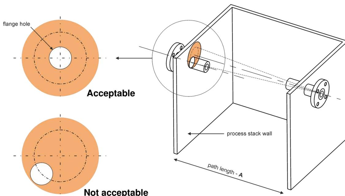
**Figure 7-4: Process flange positioning tolerance**
