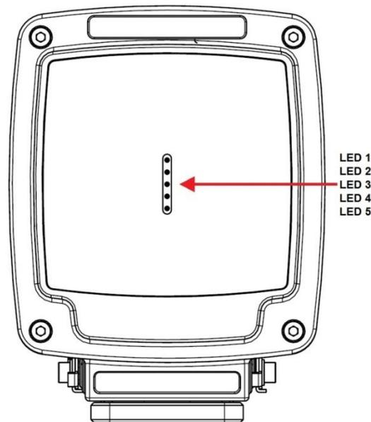
**Figure 2-5: Receiver unit indicators**
