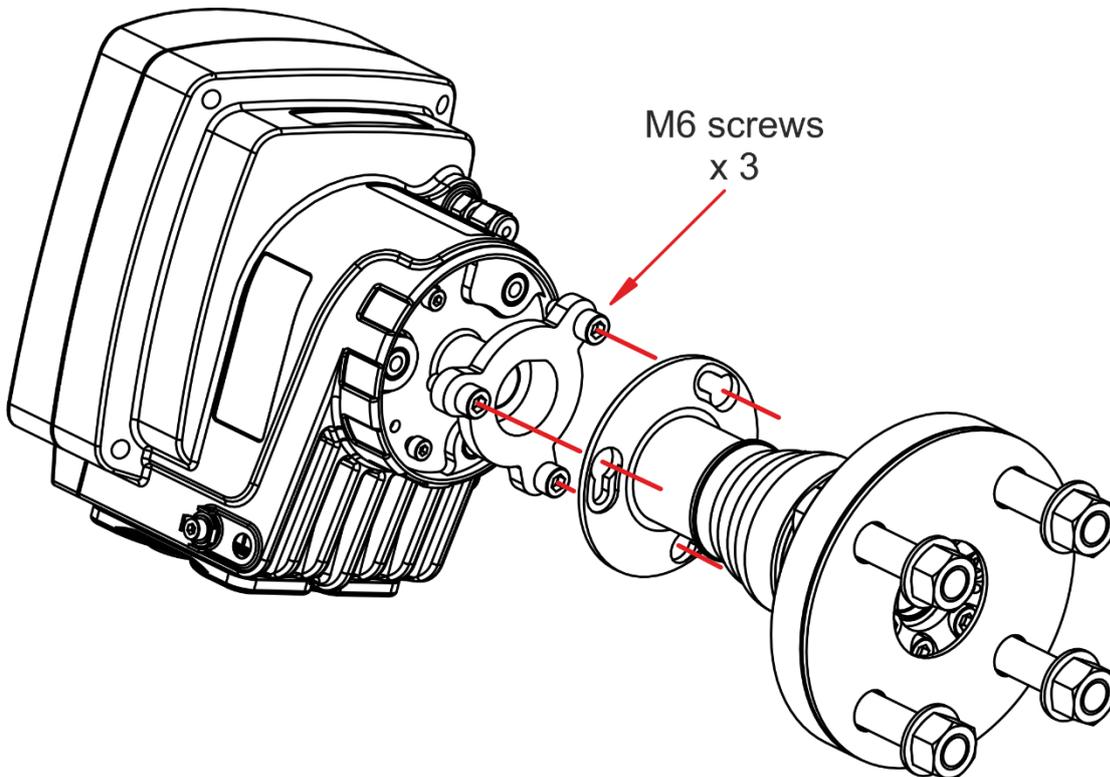
**Figure 7-11: Align M6 screws with the flange joint**
