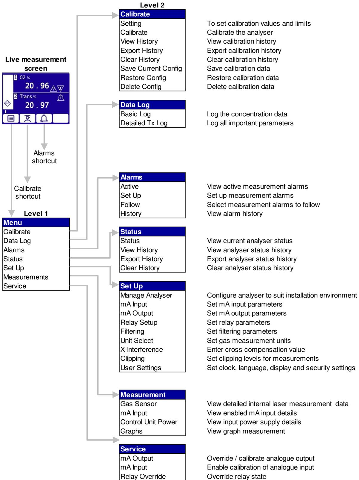
Figure 3-6: Top level menu structure
