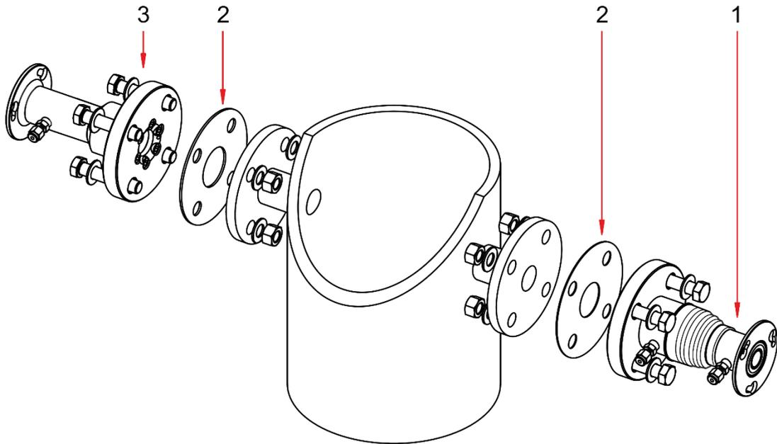
**Figure 7-9: Example of mounting / alignment assembly fitting exploded view**
