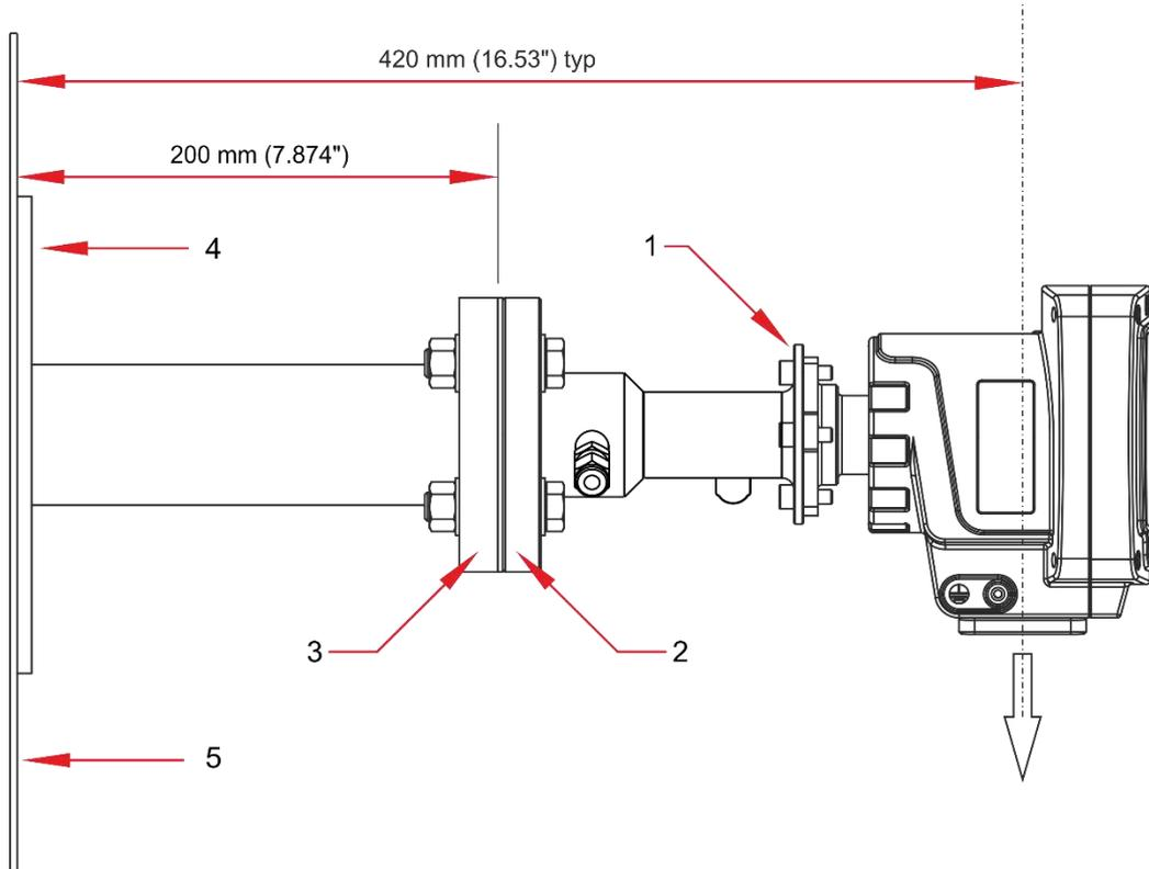
**Figure 7-6: Receiver unit mounting arrangement (example shown with fixed mount)**
