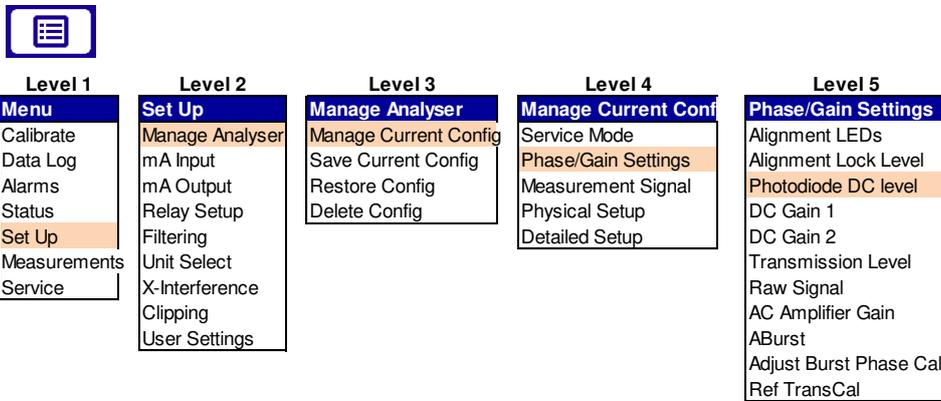
**Figure 4-31: Gain and phase setting menu**
