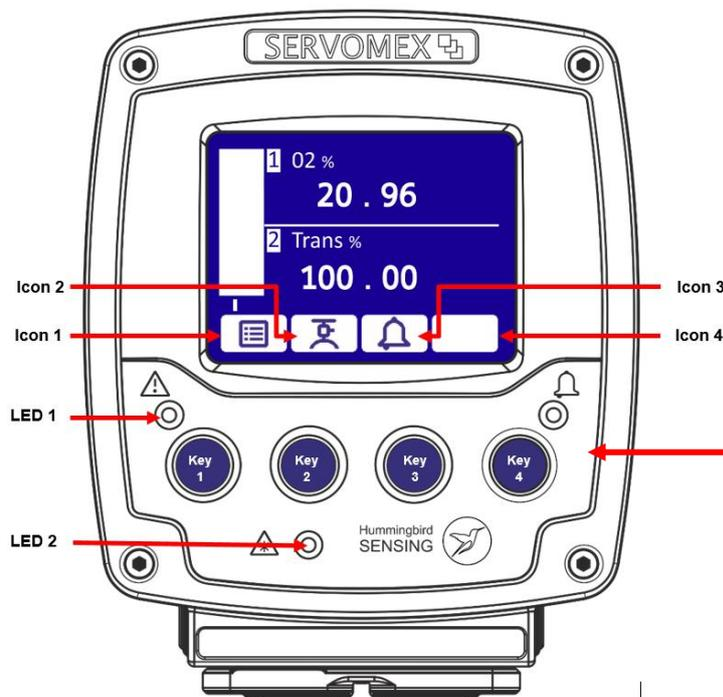
Figure 3-1: Transmitter pushbutton keys, screen icons and indicator LEDs
