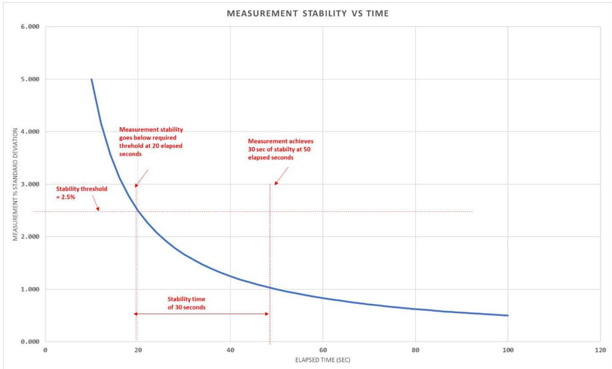
The graph above illustrates a typical scenario where a measurement is initially unstable – that is, the measured concentration or transmission is varying outside limits that would be considered normal operation. The standard deviation falls over time as the measurement stabilizes. It passes through the stability threshold level and remains below the threshold until the stability time has elapsed. At that point the measurement would be judged to be stable.
