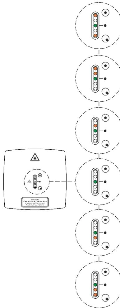
**Figure 7-29: Installation: adjust laser intensity on the photodiode**
