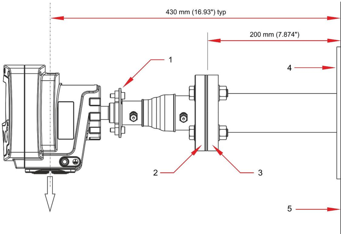
**Figure 7-5: Transmitter unit mounting arrangement (example shown with adjustable mount)**
