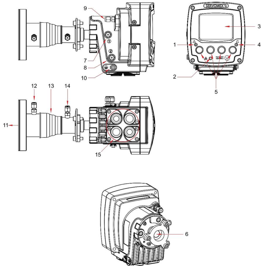
**Figure 2-3: Transmitter unit: front, rear, side and under-side views**
