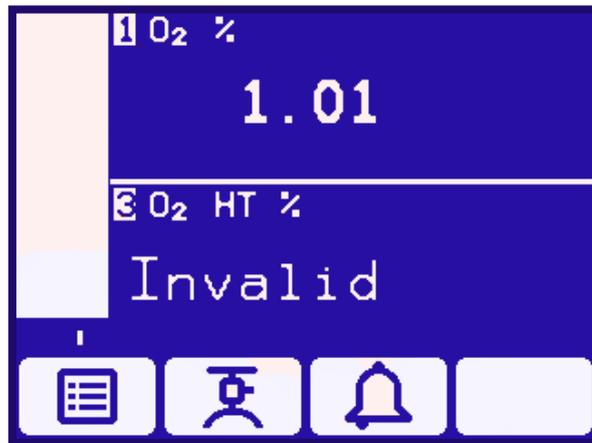
Figure 3-5: Example of an 'invalid' measurement screen
