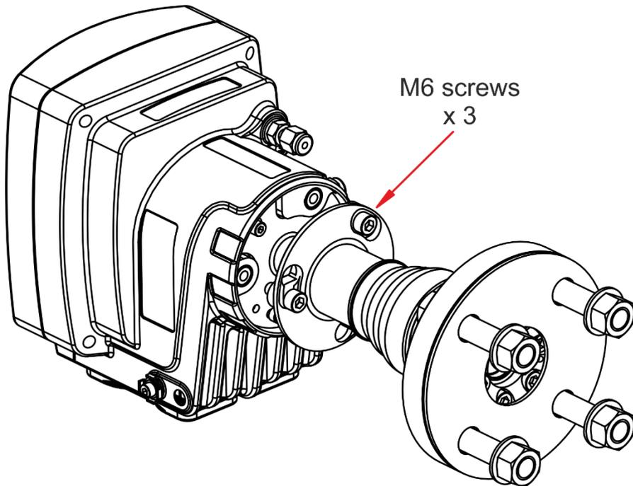
**Figure 7-13: Tighten the M6 screws**
