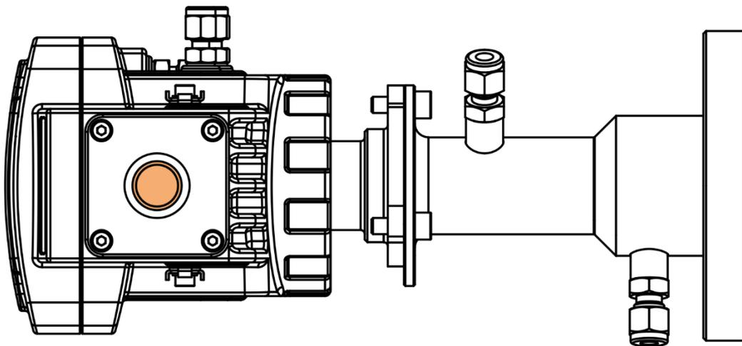
Figure 7-15: Receiver unit cable gland position
