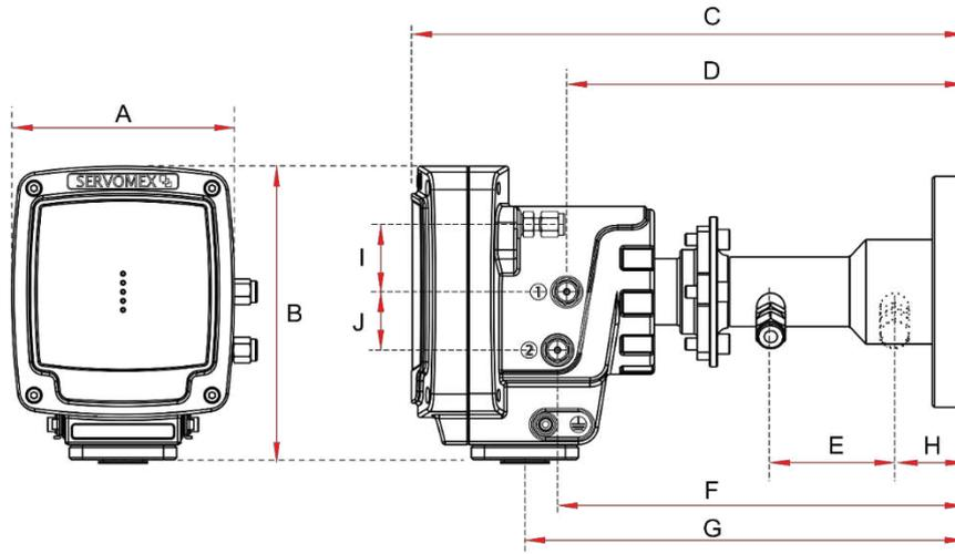
**Figure 2-7: Receiver unit dimensions**
