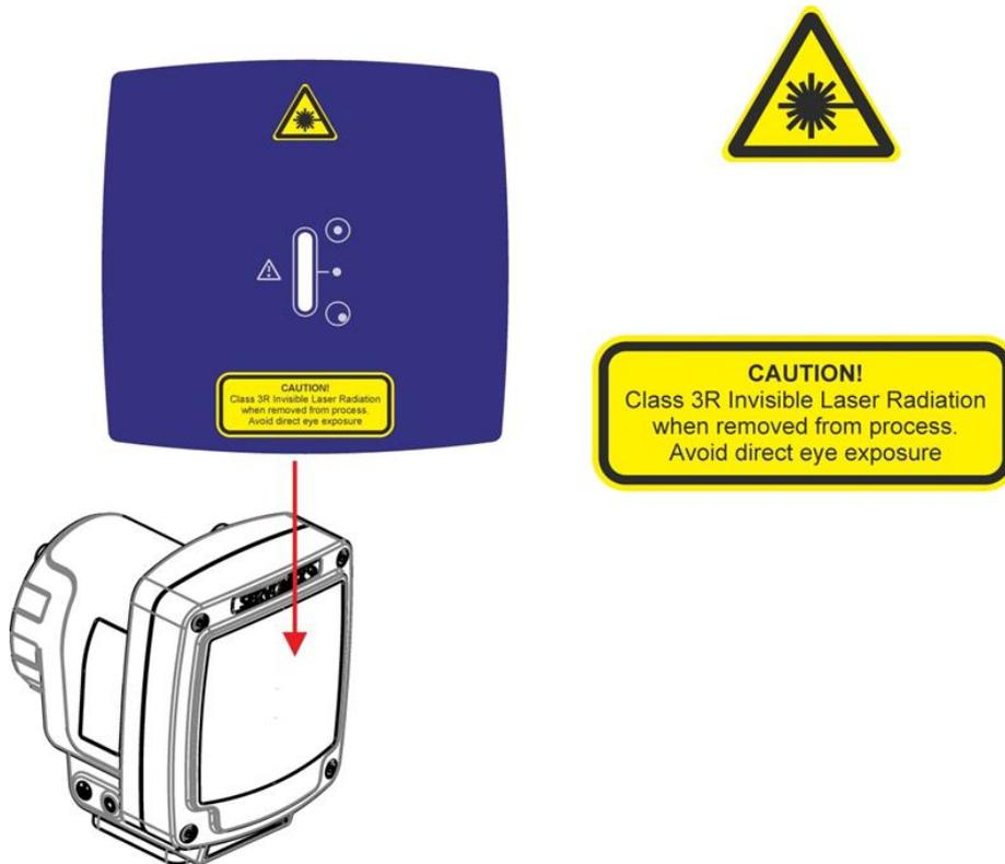
**Figure 1-4: Laser 3 Plus receiver unit laser label location**
