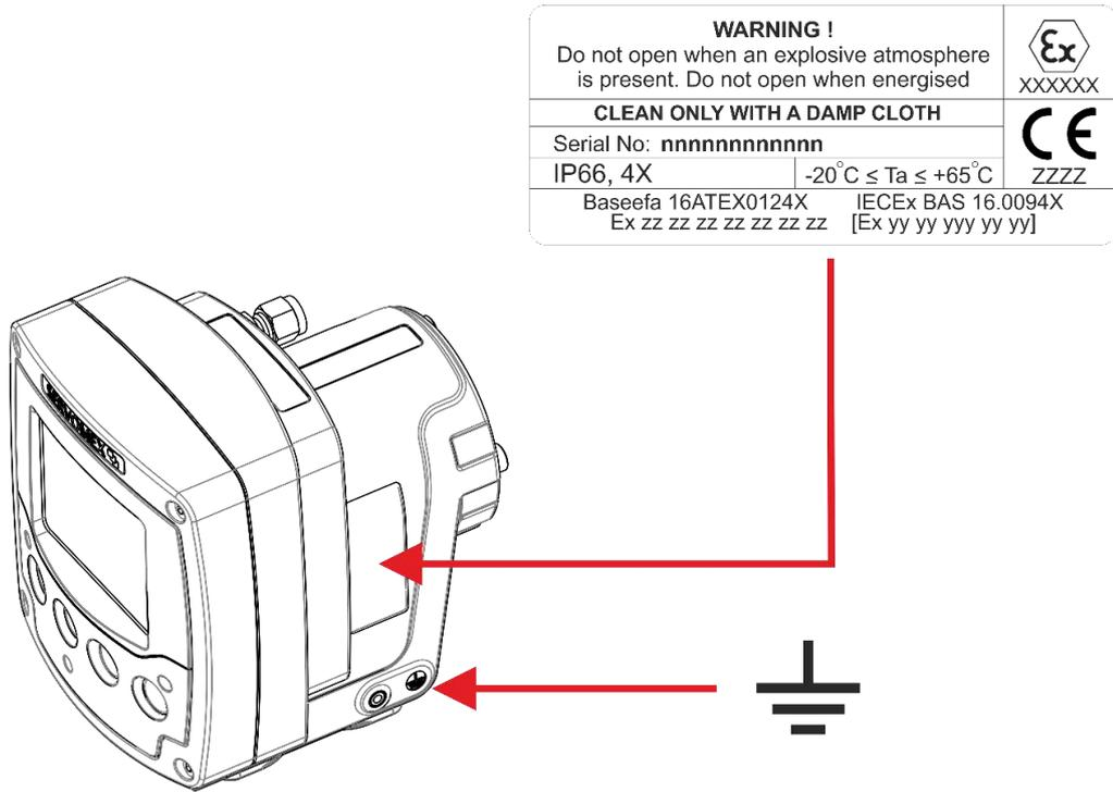
**Figure 1-3: Laser 3 Plus transmitter unit certification label
