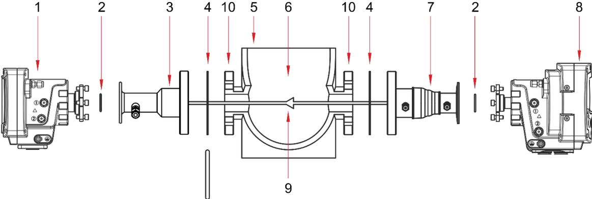
**Figure 2-1: Laser 3 Plus example installation (exploded view)**
