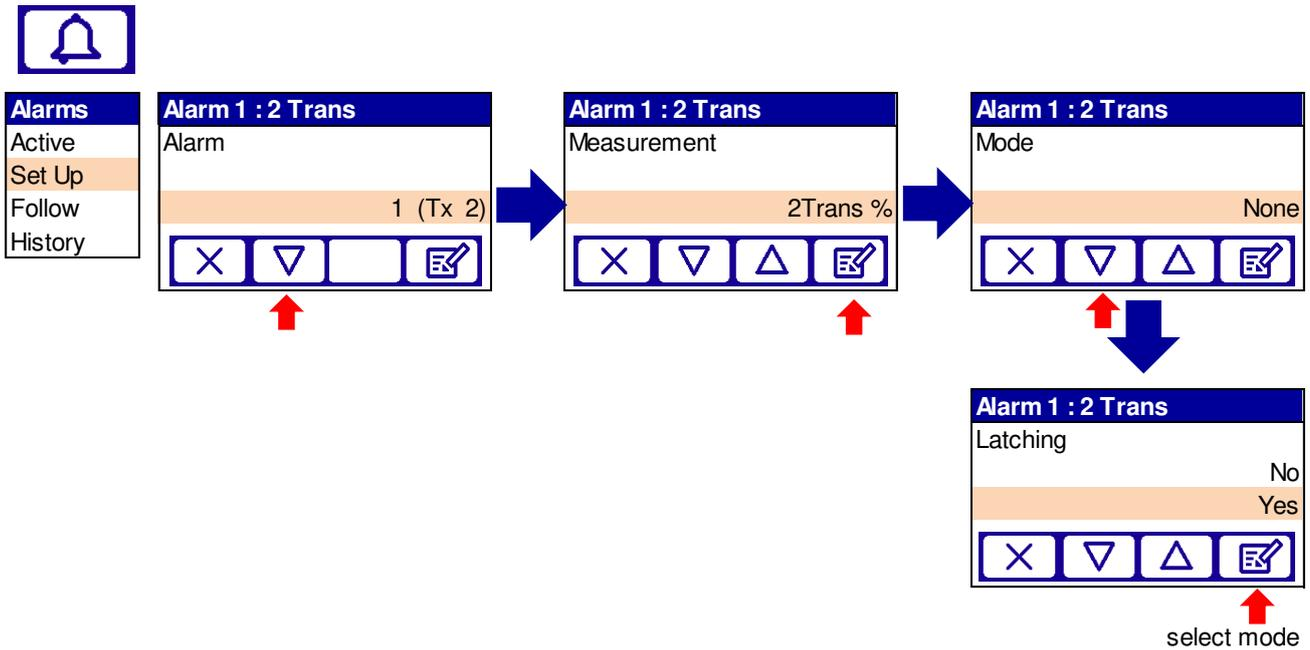
Figure 4-19: Select alarm latching mode menu
