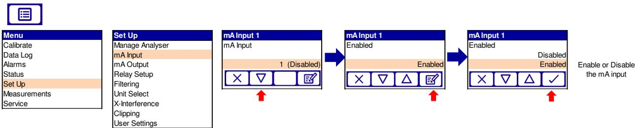
Figure 4-8: Enable or disable mA input
