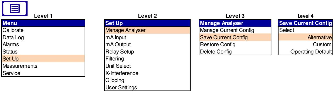
Figure 6-3: measurement sensor and environmental configuration menu
