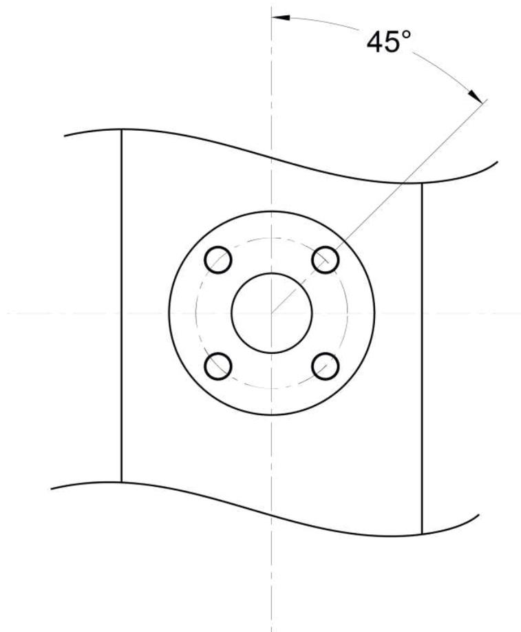
Figure 7-3: Process flange bolt arrangement (4 bolt pattern)
