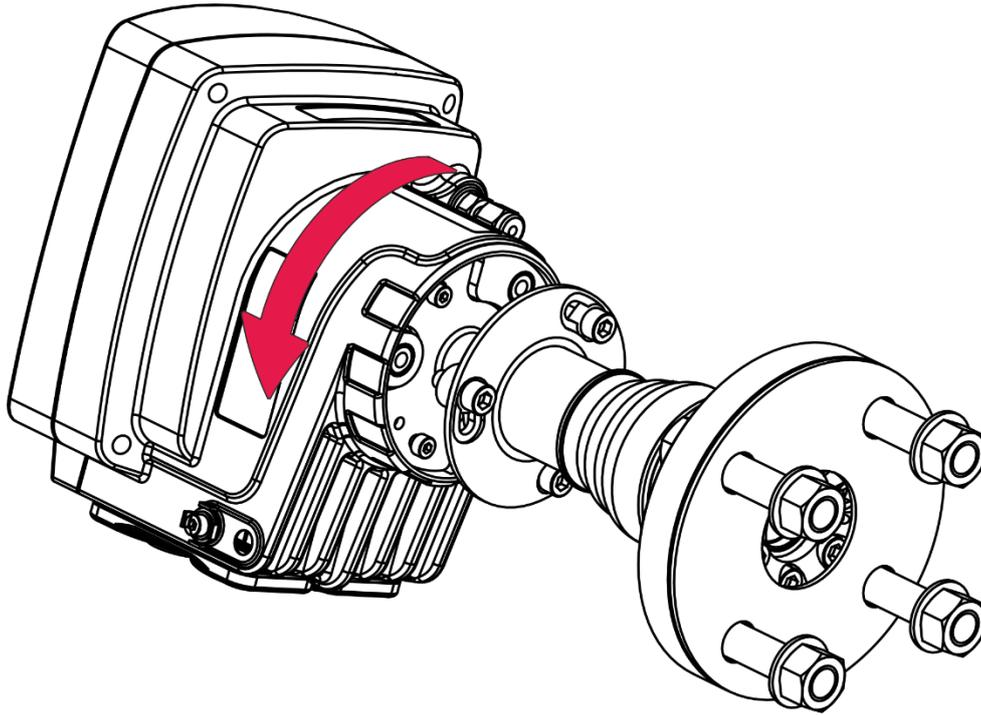
**Figure 7-12: Rotate the enclosure**
