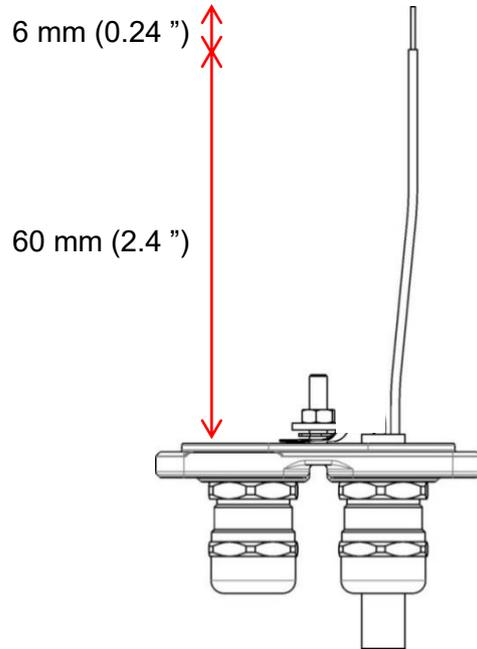
Figure 7-14: Cable strip lengths
