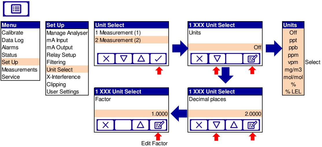
Figure 4-27: Set up units menu
