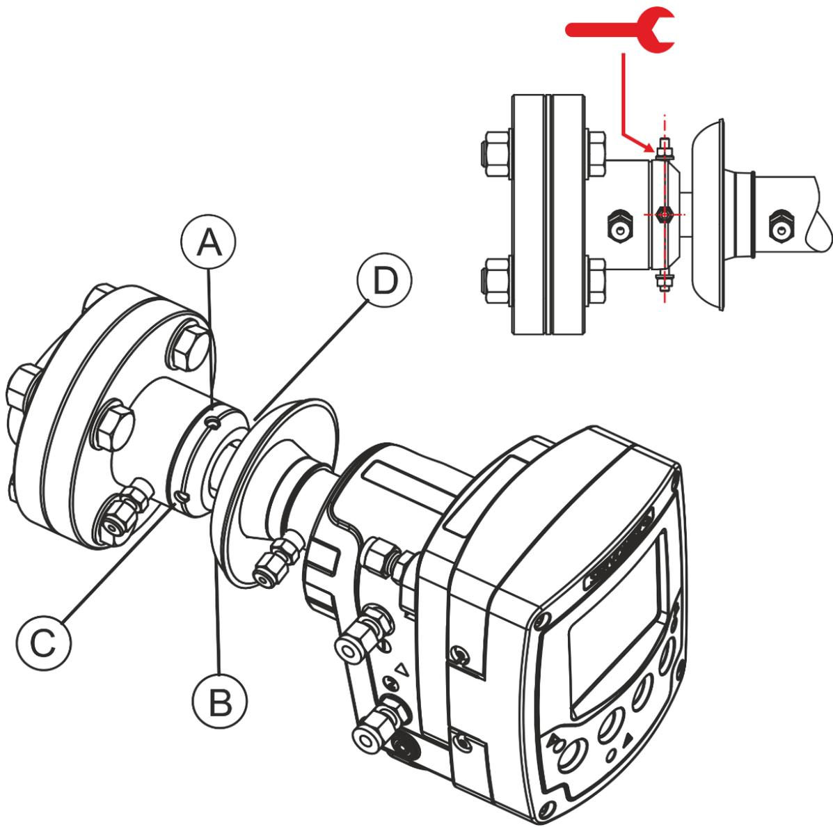
**Figure 7-25: Installation: ball-joint adjustment screws**
