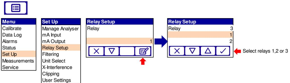
Figure 4-23: Relay output selection menu
