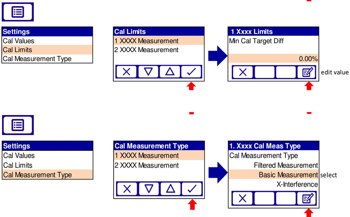
Basic cal measurement type: Uses raw transducer measurement, prior to any X-interference compensation or measurement filtering.
