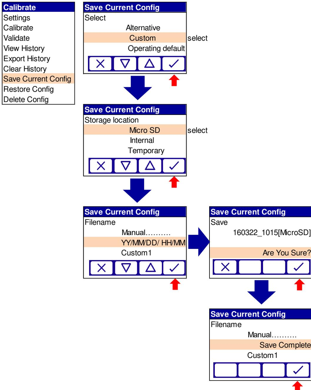
**Figure 6-5: Save calibration configuration menu**
