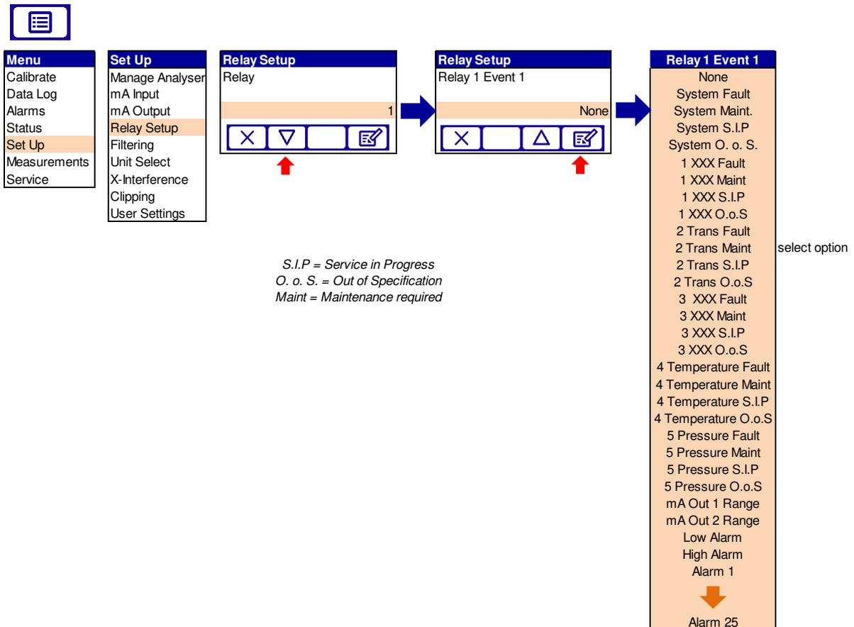
Figure 4-24: Relay output configuration menu
