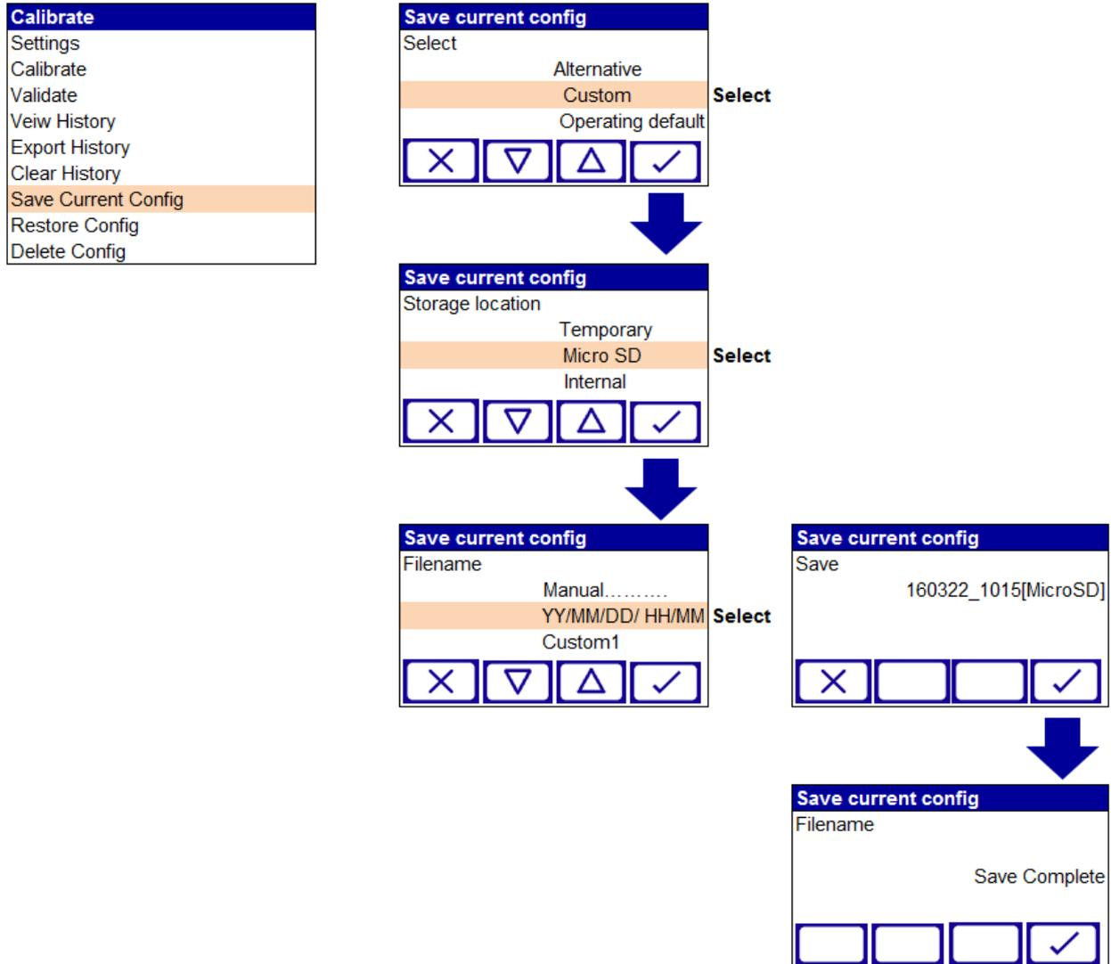
Figure 3-10: Save current calibration configuration
