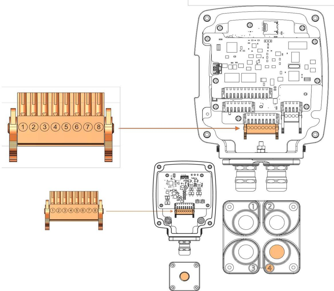
**Figure 7-19: 8-way transmitter to receiver connector**
