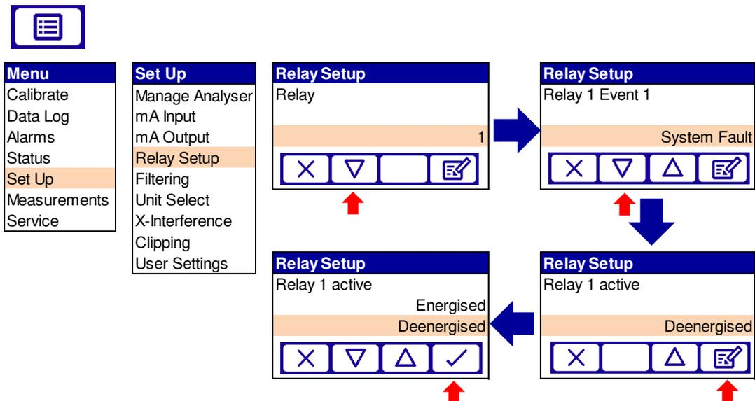
**Figure 4-25: Relay coil state menu**
