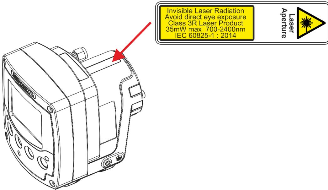
**Figure 1-5: Laser 3 Plus transmitter unit laser label location**
