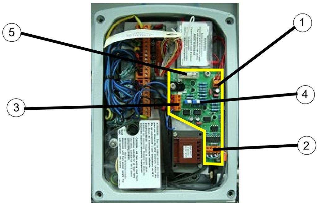
**Figure 17. Flow sensor signal amplifier board**
