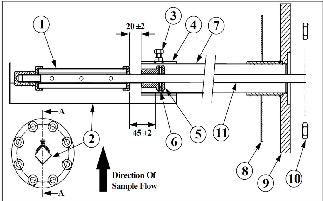
**Figure 10. Supported probe construction**
