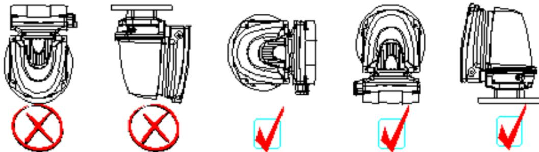
Figure 2 - Sensor Head mounting orientation
