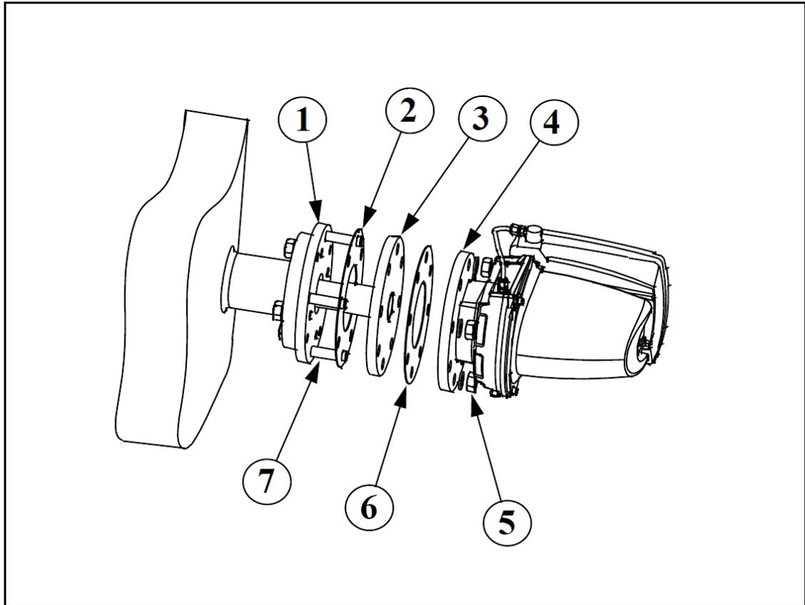
**Figure 11. Probe support tube installation**
