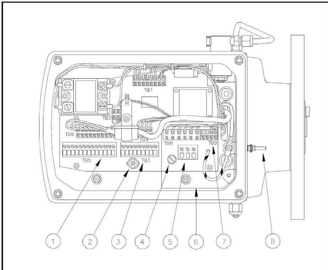
**Figure 12. Sensor head terminal enclosure detail**
