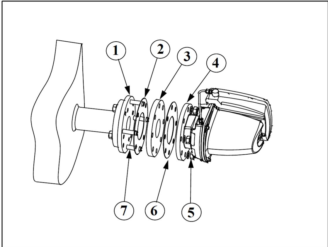
**Figure 7. Thermal spacer installation**
