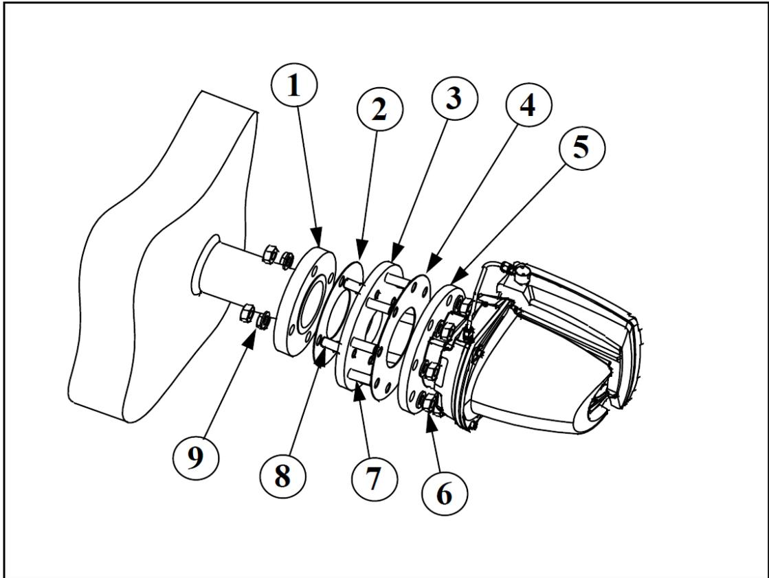
**Figure 5. Adaptor flange installation**
