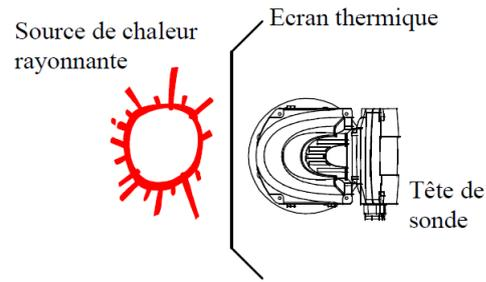
**Figure 3 – Protect from radiant heat sources and the sun**
