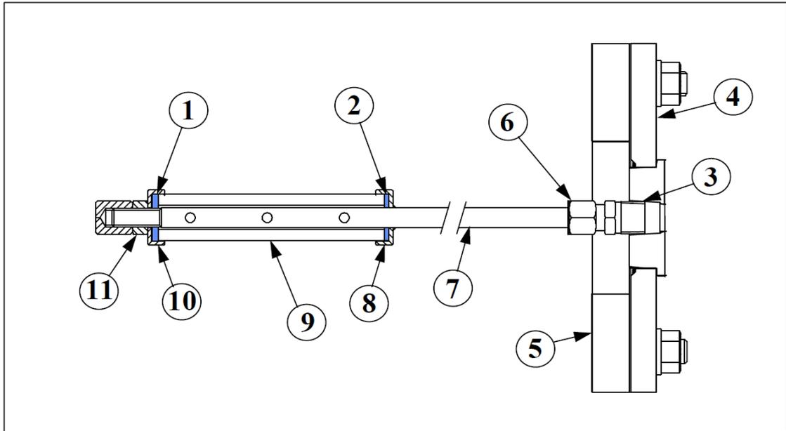
**Figure 9. Sample probe and filter construction**
