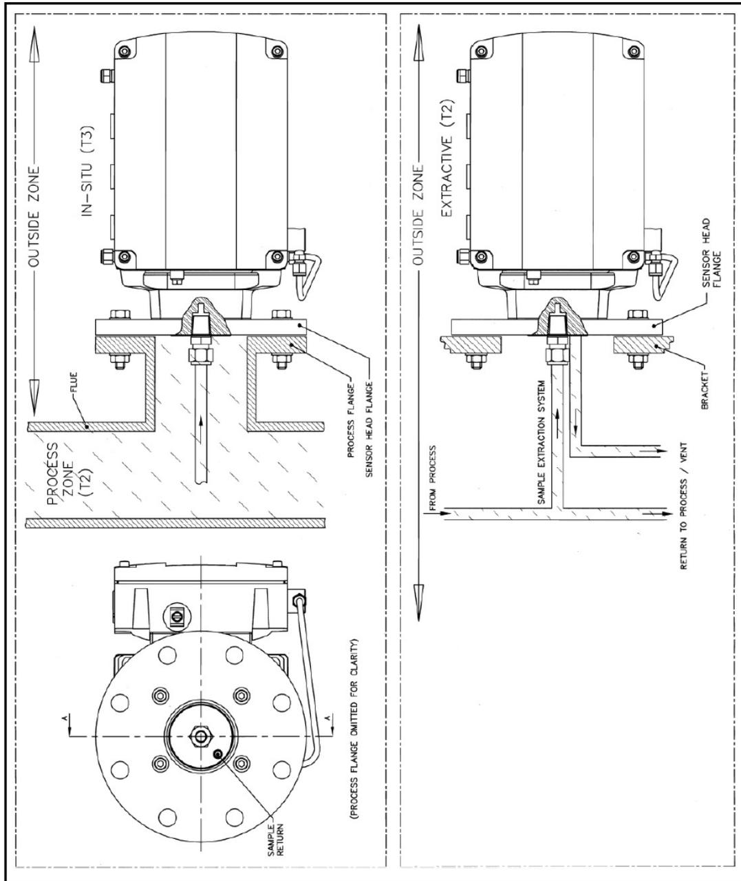
Figure 13. Typical sample arrangement
