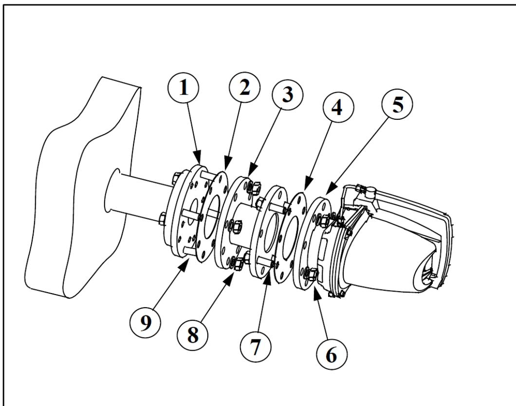
**Figure 6. High temperature stand-off flange installation**
