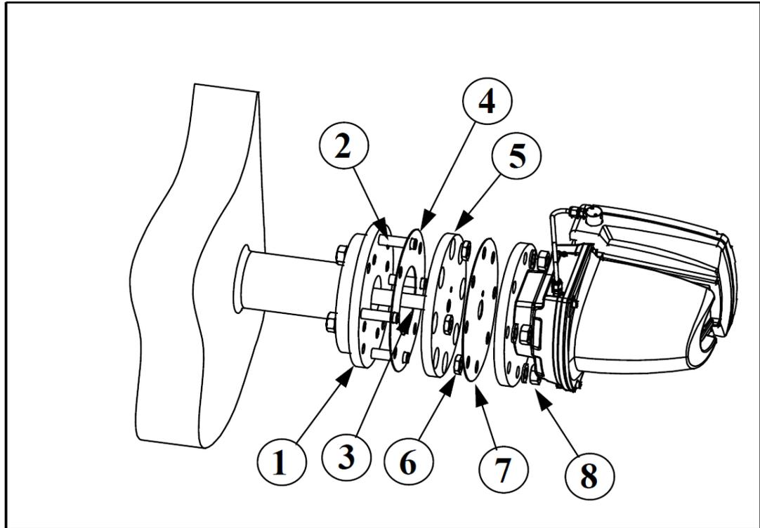
**Figure 8. Probe retention flange installation**
