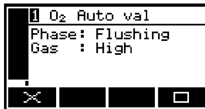
Figure 79 - The Auto val/cal status screen (flushing phase)
