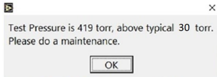
Figure 71: Pump Pressure Failure
