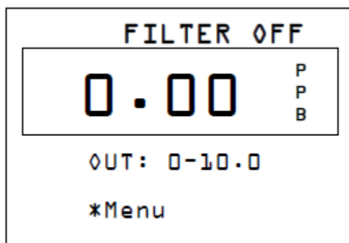
Figure 18: Averaging Filter Off Delay
