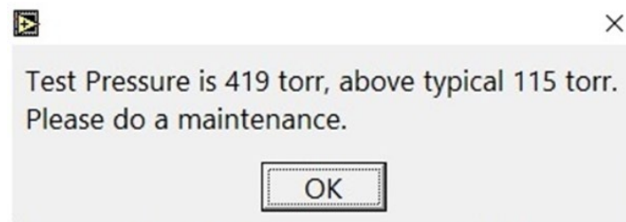
Figure 76: Pump Pressure Failure
