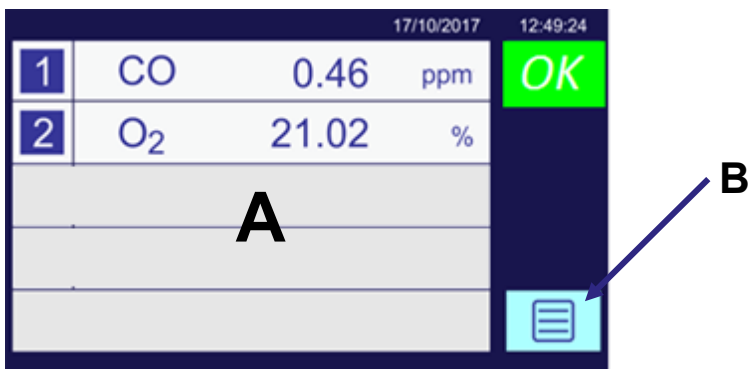
Figure 4-3: The user interface Home screen for a two-transducer configuration where (A) is the Screen and (B) indicates an Icon.
