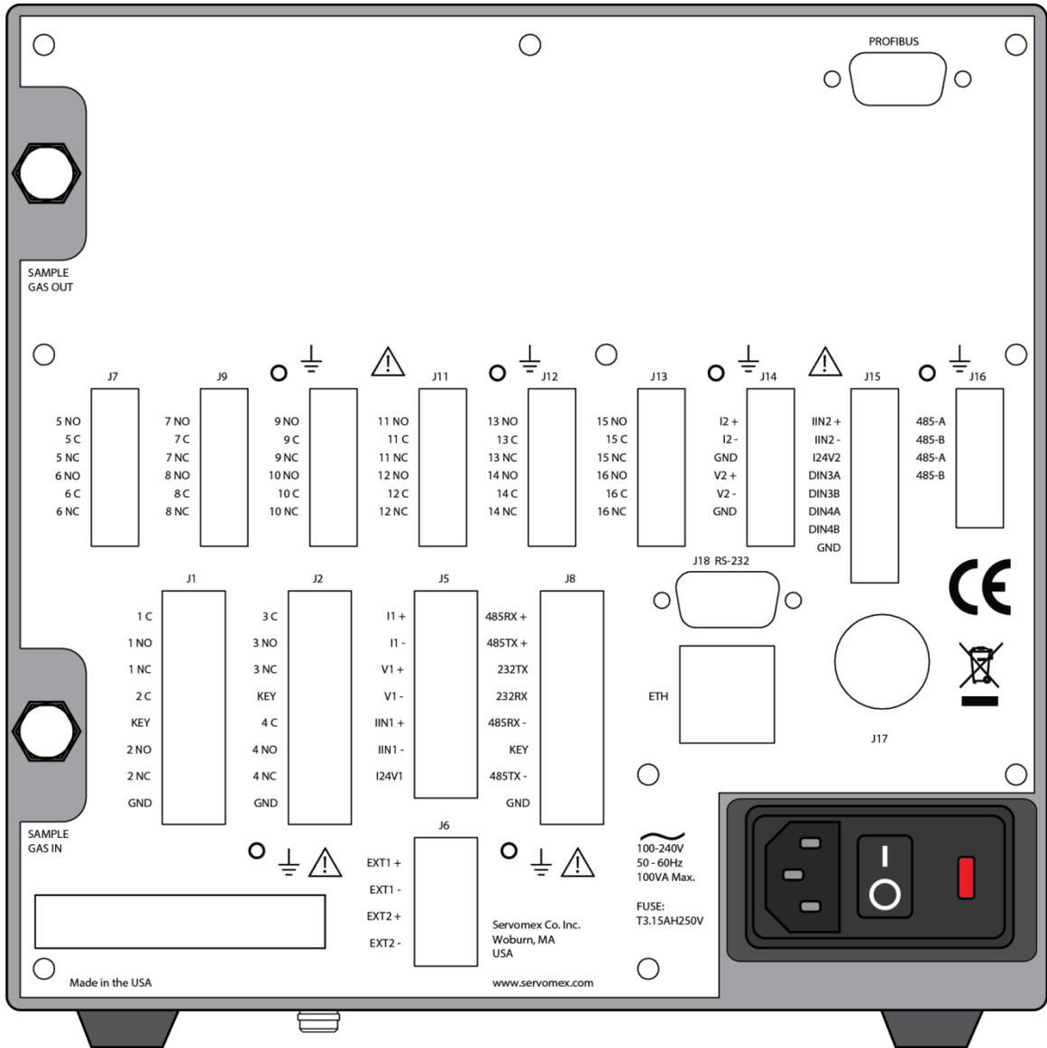
Figure 1-2: Rear of the MonoExact DF310E Gas Analyzer
