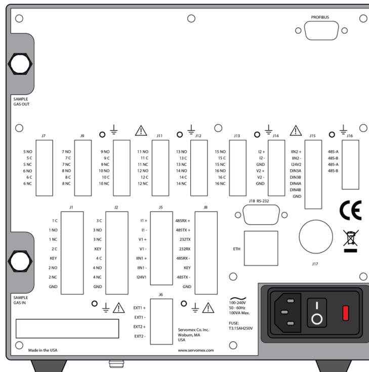
**Figure 2-1: Rear of the MonoExact DF310E Gas Analyzer**
