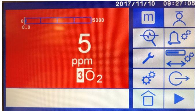
**Figure 4-6: Home screen showing O<sub>2</sub> alarm**
