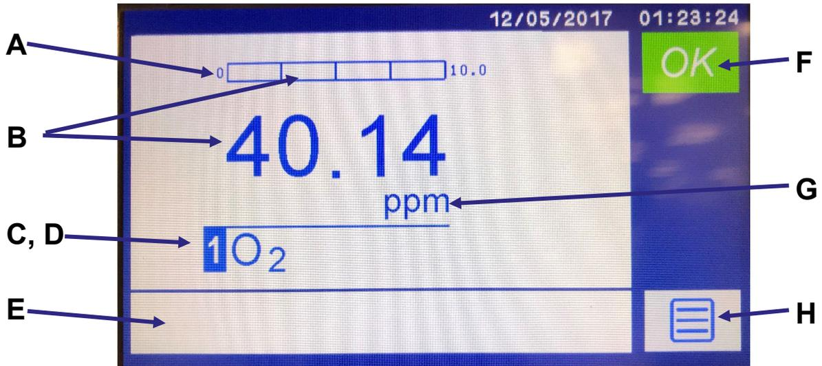
**Figure 4-4: Single Gas Home screen components**
