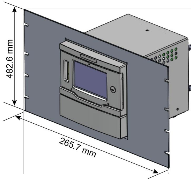
**Figure 3-3: Panel installation**
