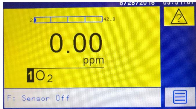
**Figure 4-7: Home screen, showing warning screen with fault description**
