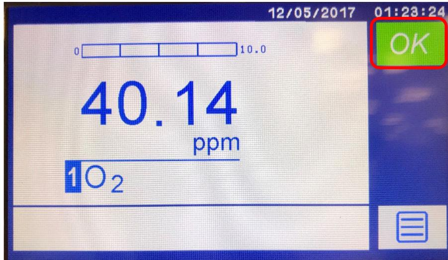
Figure 4-5: Home screen (three gas transducers)
