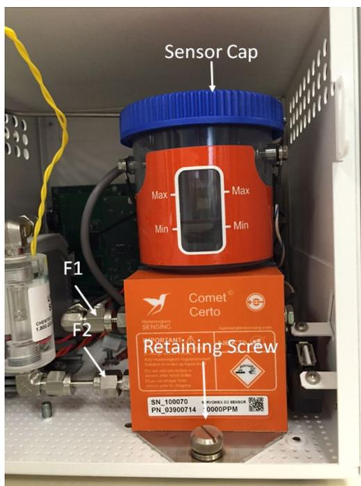
Figure 3-2: Disconnect the gas fittings
