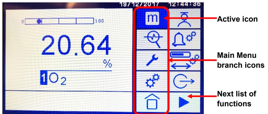
**Figure 4-2: The user interface of the Main Menu screen with the Measurement branch active.**
