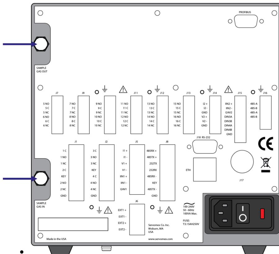
**Figure 3-1: Gas inlets and outlets on rear of the analyzer**
