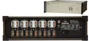
elements are maintained at  $(30 \pm 0.01)^{0}$ C in a temperature stabilized chamber. Resistance elements are electrically isolated and bonded to an aluminum block to reduce thermal gradients in the inner chamber. The inner chamber is designed to electrically shield the individual elements and an electrical connection is provided to a guard terminal at the back panel. Full specifications can be found on the Guildline website for this standard.
