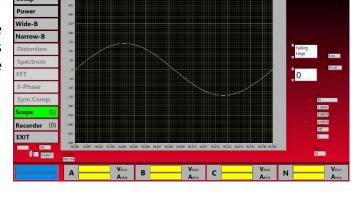
In addition to the Oscilloscope Function, there is a Recorder Function (i.e. for data logging) that captures and stores requested data. The stored data can then be further analyzed or copied onto a USB storage device.
