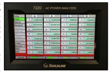
example by comparing the wideband and narrowband results a true power factor can be calculated even in the presence of a noisy signal.
