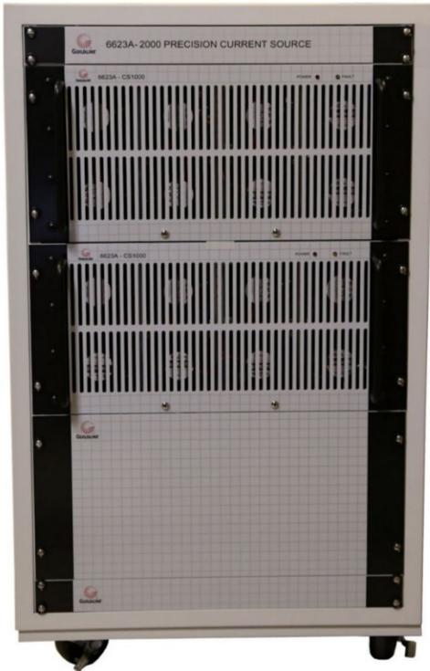
**Guildline Instruments 6623A-PCS Series** of DC Precision High Current Systems introduces new patented designs to provide the best uncertainties of any DC high current sources (i.e. typically < 5 ppm at 1000 A) and the best in modularity. The 6623A-PCS Series consists of a family of current sources, with available current outputs from 3 amperes to 10,000 amperes. The 6623A-PCS Precision Current Sources are ideal for calibrating DC Power Supplies and DC Current Shunts.
