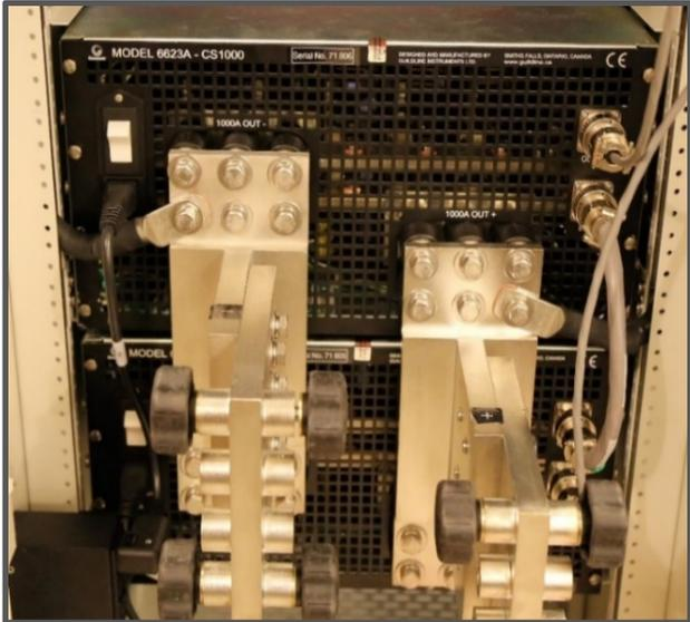
Note that MI uses third-party power supplies that are restricted to a maximum of 3000 A output current (i.e. a maximum of three of the third-party external power supplies can be placed in parallel). In comparison Guildline's 6623A-PCS comes in standard configurations up to 10,000 A.
