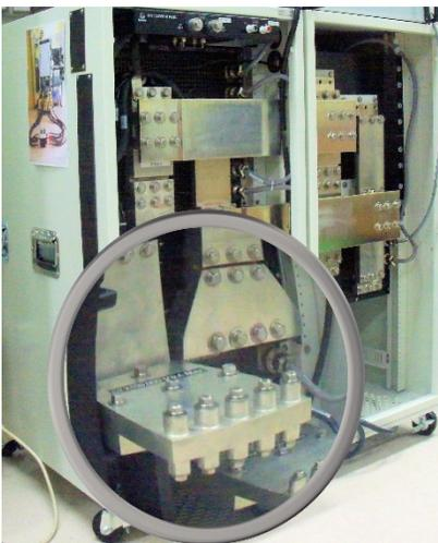
**How good is the 6623A-PCS?** Measurement results from a 1000 Ampere Inter-comparison of two NMs (Test Results shown below right) came within 5 ppm of each other. One setup was a Guildline 6623A-PCS/4000A System with our 66259 Controller. This system is shown to the left.
