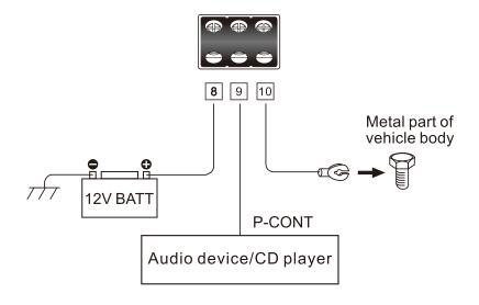
Controls & connector Diagram
