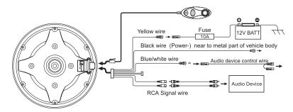
With control via the Low-Level Inputs [also referred to as RCA Inputs], connect the blue color remote wire from the DQC-582T to the vehicle's head unit so DQC-582T will be turn on and off with systems.
