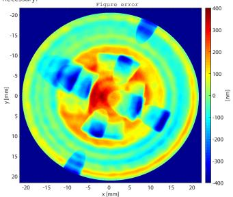
The figure shows the measured surface defects as well as the form deviation of an asphere with MRF footprints.
