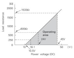
Note: For communication with  $HHC^{\mbox{\tiny (1)}}$  (Model: FXW), min. of 250 $\Omega$  is required.
