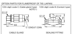
NOTE 1) IN CASE OF 10TH CODE "C", ¢11 CABLE IS SUITBLE. NOTE2) WHEN THE 7TH DIGIT OF THE CODE SYMBOLS "H,M,T" NOTE3) THE PRESSURE CONNECTOR IS LOCATED ON THE DOWN SIDE SURFACE OF THE DETECTOR, WHEN THE VENT/DRAIN PLUG IS ATTACHED ON THE UPPER SIDE OF THE DETECTOR (WHEN THE 21ST DIGIT OF THE CODE SYMBOLS : C, P).
