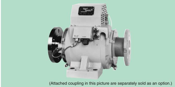
The DD Series is high performance of SS Series, which can measure the larger capacity torque at higher speed. Model DD-505 to DD-108 are mostly suitable for the torque measurement with heavy load. The double bearings provide three to five times the strength of the DSTP Series under radial and thrust load. Further, it can be connected directly with propeller shaft which does not need the intermediate coupling and save space as well. Oil drop lubrication unit is required.
