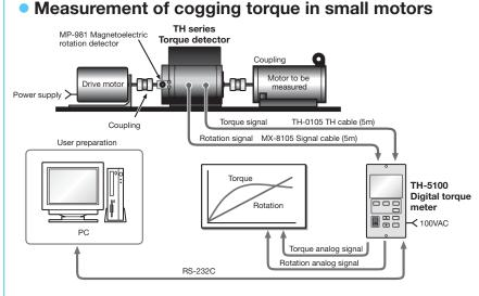
The TH series torque detectors measure cogging torque in small motors with fast response capability.
