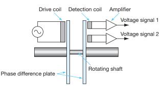
The above drawing shows the interior structure of the torque detector. It is configured with a rotating shaft, phase difference plates, where a drive coil and detection coils are located face to face. A magnetic signal that flows from the excited drive coil to the phase difference plates is converted into an electric signal by the two detection coils.
